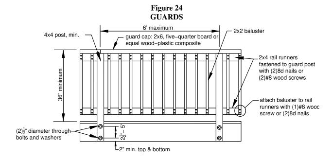
**Guard posts.** Guard posts must be attached to the deck structure in accordance with all of the following: Notching guard posts, as shown in Figure 25, is prohibited.
