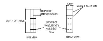
ATTACH TOP OF KEY-BLOCK TO INSIDE FACE OF RIBBON BOARD WITH 2 - 10d (0.131" x 3") THROUGH NAILS AND 2 - 10d TOE-NAILS. ATTACH BOTTOM OF KEY-BLOCK TO SILL PLATE WITH 4 - 10d TOE-NAILS
