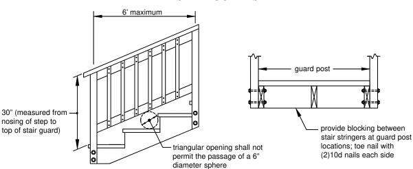
**Stair handrails.** A flight of stairs with more than 3 risers must have at least one handrail that complies with all of the following:
