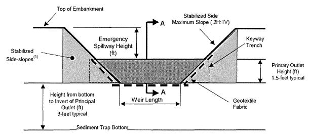
Figure 1: Sediment Trap Outlet Detail
