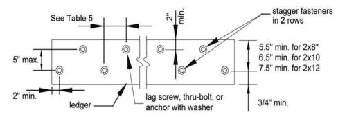
See Figure 11 for band-board fastener spacing.
