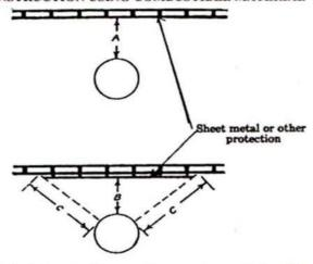
"A" Equals the required clearance with no protection, specified in s. SPS 323.045 (4) (b).
