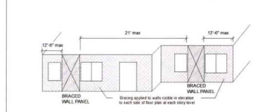
\*A braced wall panel can be anything from one-half to one brace panel.
