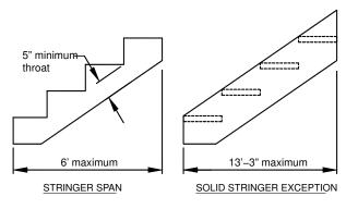
**Tread and riser material.** Treads and risers must comply with all of the following:
