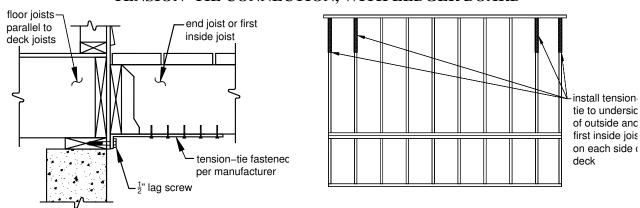
**Tension-tie requirements.** Tension ties, if used instead of perpendicular bracing as described above, must comply with all of the following, but are not permitted for free-standing decks:
