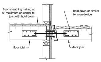
**Hold–down tension devices.** Hold–down tension devices, if used instead of perpendicular bracing as described above, must be provided in at least 2 locations per deck, and each device must have an allowable–stress–design capacity of at least 1,500 pounds.
